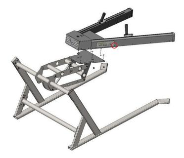
C) Attach the gas spring activation lever right below the green on/off switch with (2) #8-32 lock nuts (finger tight only). DO NOT ENGAGE THE GAS SPRING ACTIVATION LEVER UNTIL THE MACHINE IS ASSEMBLED.
